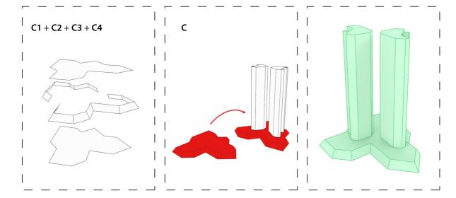
Now, you add the parts of the base plate together into one piece.
