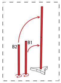
Rotate the core parts to create cylinders and glue them on top of each other.
