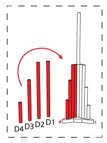
Complete the second side by gluing cylinders next to each other.
