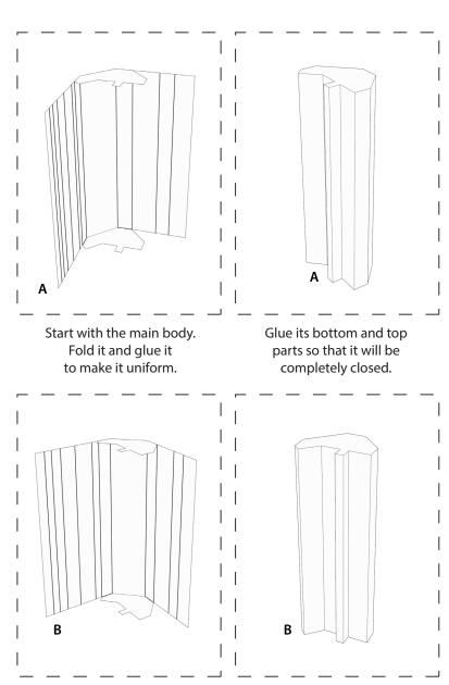
Then, repeat the process with the twin body. Fold it and glue it to make it uniform.
